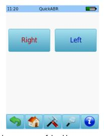
A calibration will be performed prior to measurement. A green light indicates successful calibration.
