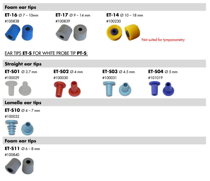
Please make sure that the selected ear tip properly fits into the ear canal. Once inserted, the ear tip should remain in the fitted position. Before inserting a foam tip, squeeze the foam. After inserting the foam tip wait a few seconds to allow the foam to extend. If leakage is indicated on the device screen when starting a test, reposition the ear tip in the ear canal and/or try another ear tip size or shape before restarting the test.
